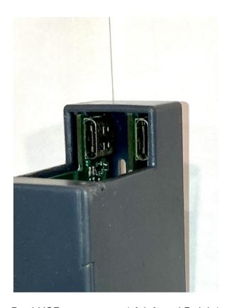
Dual USB connectors ( A left and B right)
